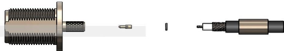
2) Slide the insulator over the centre core then solder or crimp the pin onto the centre core. Next slide the pin into the body until fully located in the integral contact, ensuring that the cable braid is on the outside of the connector mandrel.
