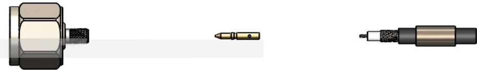
2) Crimp the pin onto the centre core and slide the pin into the body, ensuring it is captive and that the cable braid is on the outside of the connector mandrel
