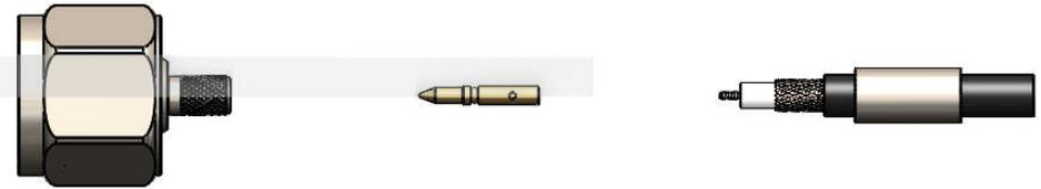
2) Crimp the pin onto the centre core and then push into the body, ensuring that the cable braid is on the outside of the connector mandril and that the centre pin is fully located.
