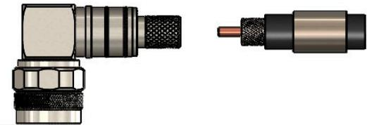
2) Insert the cable into the body, ensuring that the cable braid is on the outside of the connector mandrel and that the centre core is fully located
